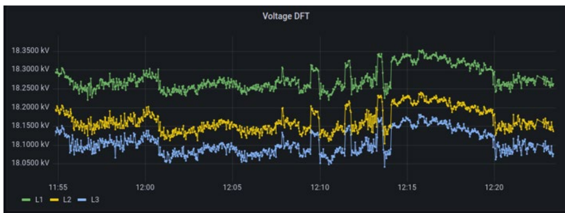
Figure 27 Voltage magnitude profiles obtained from three edgePMUs for 25 minutes
