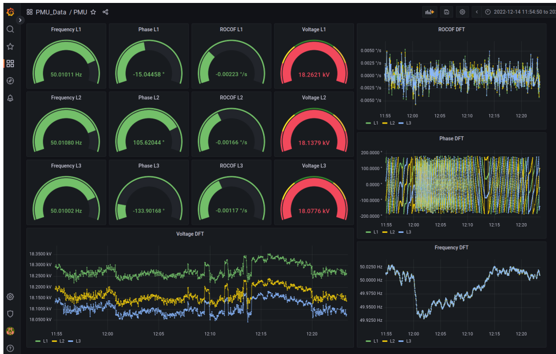
Figure 26 Dashboard for the visualization of the edgePMU data
